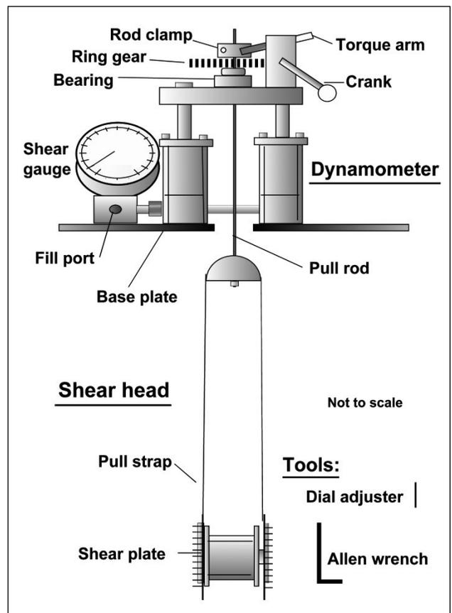
Figure 3. Borehole Shear Test Schematic.
